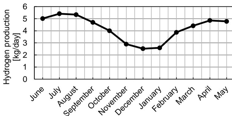
considers the real operating conditions of the ELY, metrological conditions and maintenance issues. The model is validated with experimental data gathered during the demonstration phase of the project ELY4OFF (FCH JU n°700359) [12] from March to September 2019. Since no data is available for a full calendar year, the model is used to extrapolate hydrogen production in the missing months.
