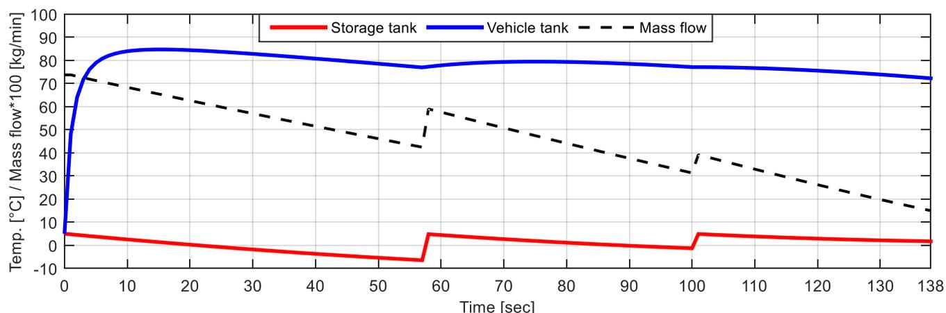
Figure 4. Temperature (red and blue solid lines) and mass flow (dashed line) evolution during a refuelling event
